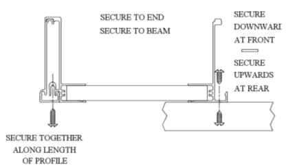
Lift a further pre-assembled panel on to the roof and locate onto the previously fixed Aluminium profile. Secure as above using fixings supplied.
